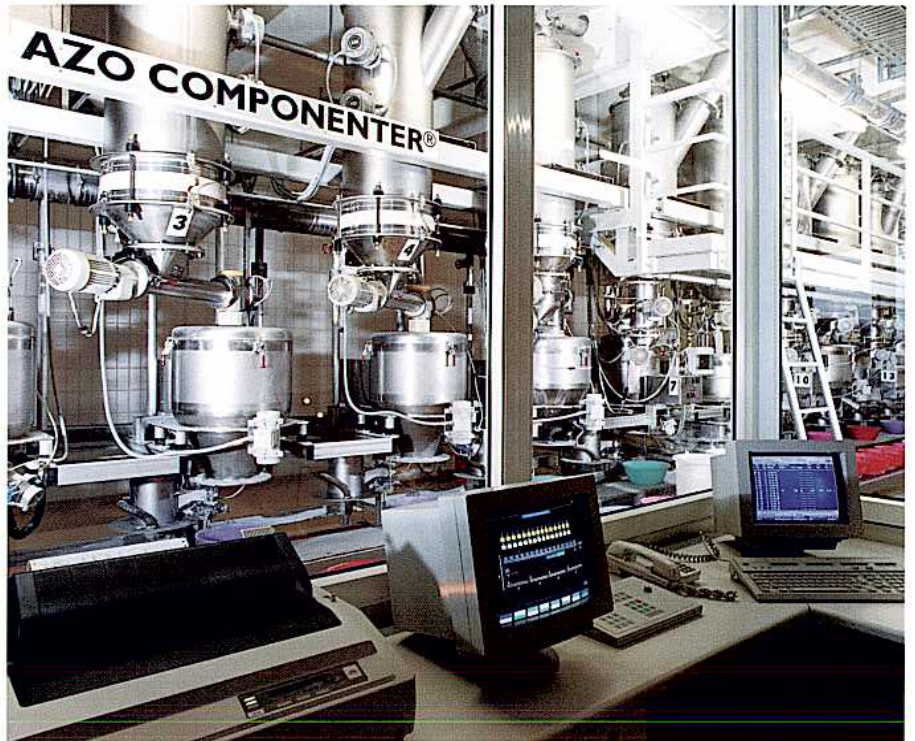
Central process control and graphic display system
