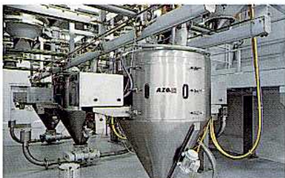
Collecting hopper can be moved for cleaning
