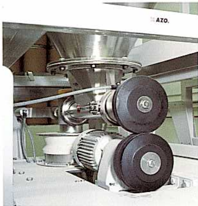
Frictional wheel for metering screw
