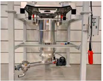
Big bag connection system with  $\varnothing$  500 hopper with mounted dosing screw (not part of the modular system)
