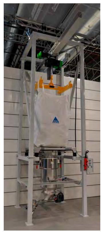
modular discharge station for big bags with mounted dosing screw (not part of the modular system)
