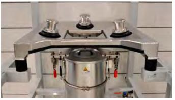
Support hopper with vibrating discharge aid and massager device
