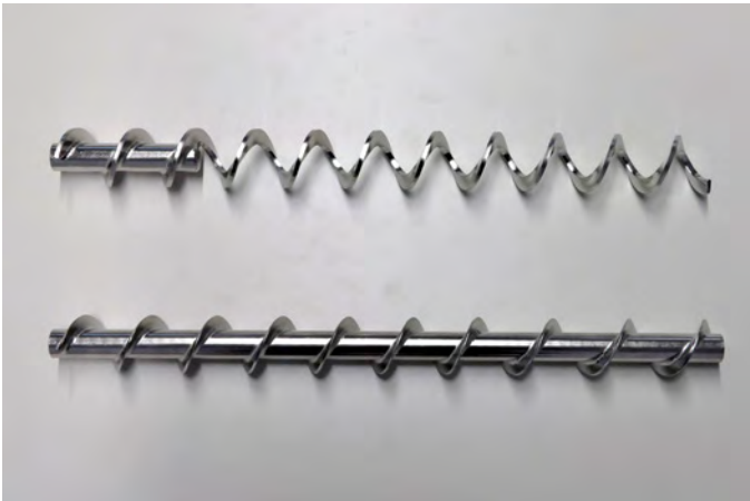
Following screw variants are available for single screw dosing systems: Spiral screw (top), full flight screw (bottom)
